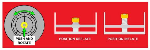
Now, attach the pump's hose to the valve by turning it clockwise, and inflate the board up to a maximum pressure of 14 PSI (1.0 bar).
