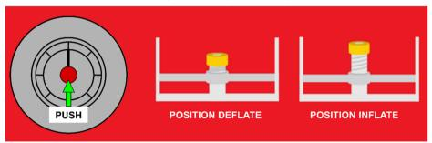
Next, attach the pump's hose to the valve by turning it clockwise, and inflate the main board up to a maximum pressure of 14 PSI (1.0 bar).
