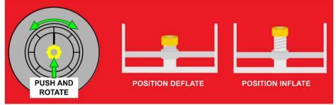
Now, attach the pump hose to the valve by turning it clockwise and inflate the board up to a maximum pressure of 14 PSI (1.0 bar).
