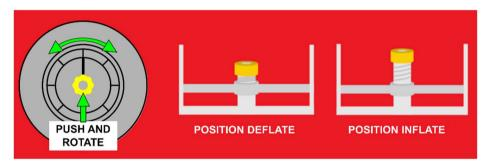
Next, attach the pump's hose to the valve by turning it clockwise, and inflate the board up to a maximum pressure of 10 PSI (0.7 bar).
